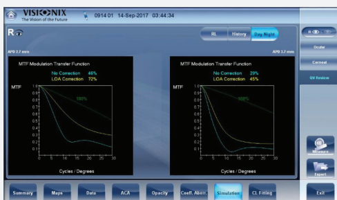
Objective day and night refraction measurements. Analysis of aberrations with Zernike coefficients
